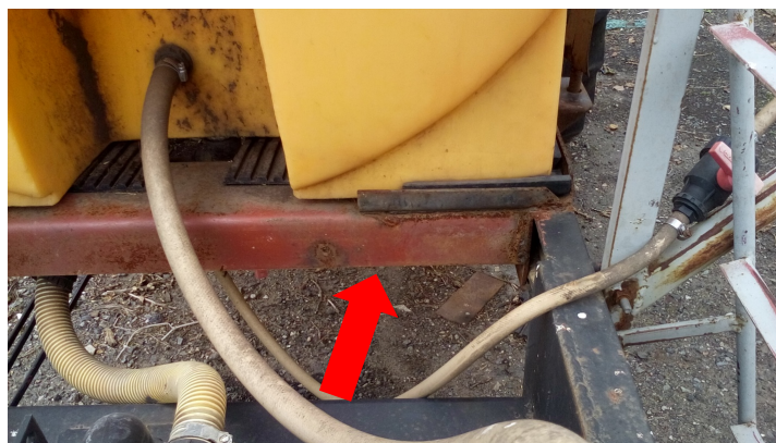
Fig. 10. Installed additional traverse
